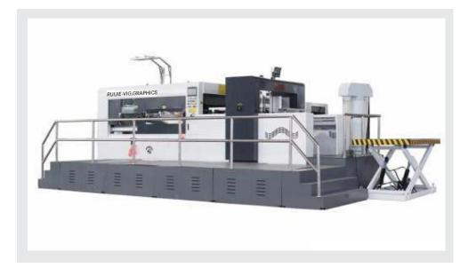
Suitable for die-cutting and embossing of paper boards and multi-flute cartons.
