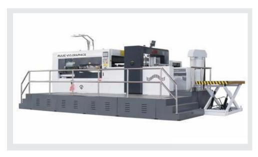
Suitable for die-cutting and embossing of paper boards and multi-flute cartons.
